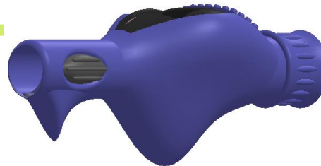
The second side is slipped into place with the integrated snaps.
