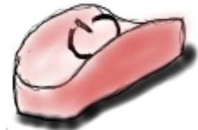
Power button on top to avoid accidental power on/off
