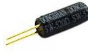
Tilt Switch to measure device activity
